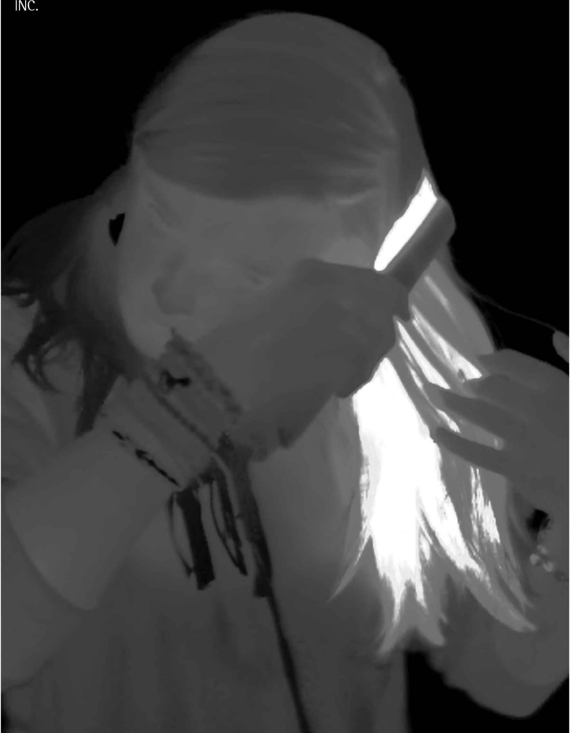
Figure 63: Thermogram of a woman using a flat iron to apply heat to straighten her hair. Thermography records surface temperatures by detecting the long-wavelength radiation emitted by an object. Here, the color-coded temperature scale runs from white (warmest) through yellow, red and purple to black (coldest).©TONY MCCONNELL/PHOTO RESEARCHERS, INC.
